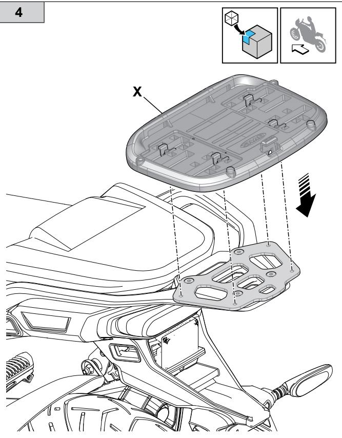
**GB** Connection plate (X) supplied with the 37-litre top box. For assembly, see the relative instructions in the top box.
